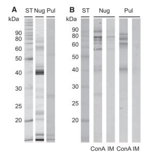
**Fig. 3.** Gel with 10% polyacrylamide (SDS-PAGE) silver-stained (A) and affinity blotting with lectin ConA and inhibition by saccharide inhibitor (B). ST—marker; Nug—*C. nubeculosus* (SGE); Pul—*C. pulicaris* (SGE); ConA—biotinylated lectin concanavalin A; IM, inhibitory mannose.
